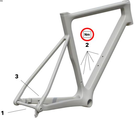
! Maximum torque for bottle cage bolts: 4 Nm
