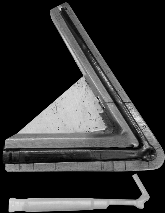
Pre-formed rear triangle NDS before curing & CS-Dropout mandrel.
