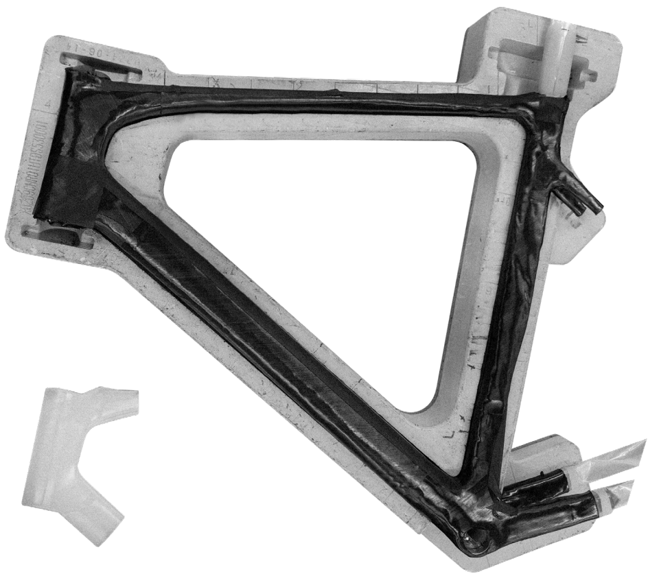
Pre-formed main triangle before curing & HT mandrel.
